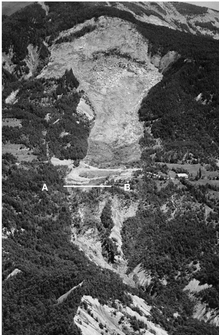
Fig. 1. Aerial view to the North of the La Valette landslide, near Barcelonnette (French Alps). AB: the line where velocities were measured.
